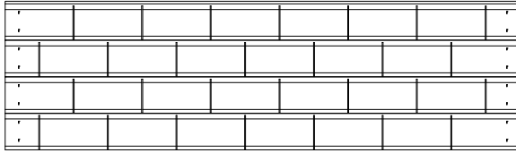
RP1 | LOWER ROOF PANEL - W2A03184 (x2) | 1 3/8"x13"x44 7/8" (35x329x1140)
